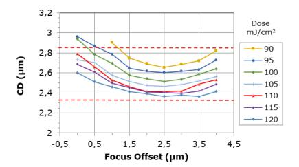
Mask CD: 2.6µm lines @ 1:1 pitch
