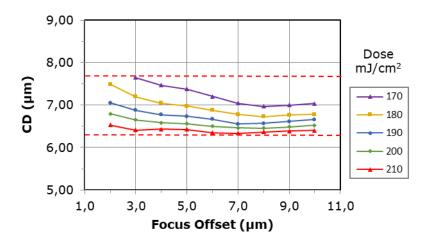
Mask CD: 7.0µm lines @ 1:1 pitch
