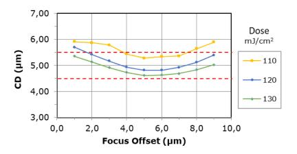
Mask CD: 5.0µm lines @ 1:1 pitch
