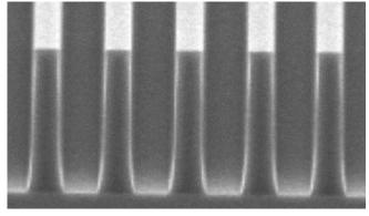
2.4µm lines in 10µm thick AZ 12XT 110mJ/cm2 Exposure AZ 300 MIF Develop (120s)
