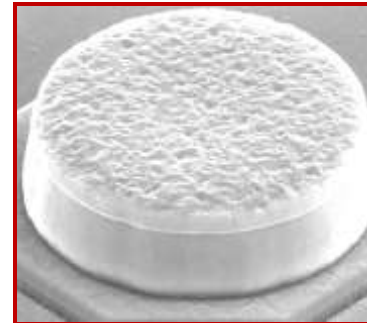
Bottom die with thin SnAg coverage with different Aspect ratios
