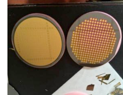
before and after positive resin stripping on aluminium pad
